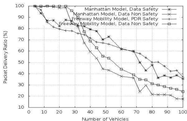
Fig. 8. Variation of packet delivery ratio with number of simulated vehicles
