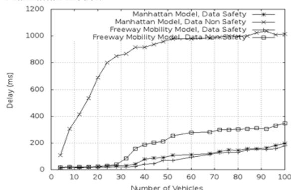
Fig. 7. Variation of delay with number of simulated vehicles
