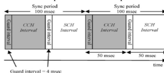
Fig. 3. Allocation CCH interval and SCH interval [11]
